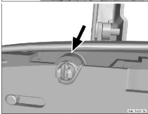
Close the opening flap and make sure that the mark on the toothed segment (arrow) is pointing vertically up.
