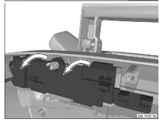
Slip your hand between case shell and latching mechanism and pull gently down to disengage it from the holding points: the mechanism disengages with an audible click.
