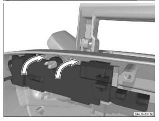
• Push the mechanism onto its holding points.
